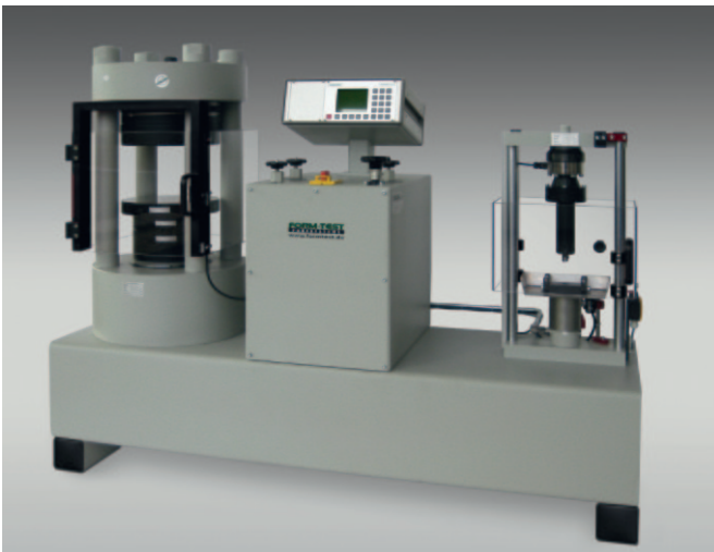
special design with bending testing for prisms (cement/mortar)
